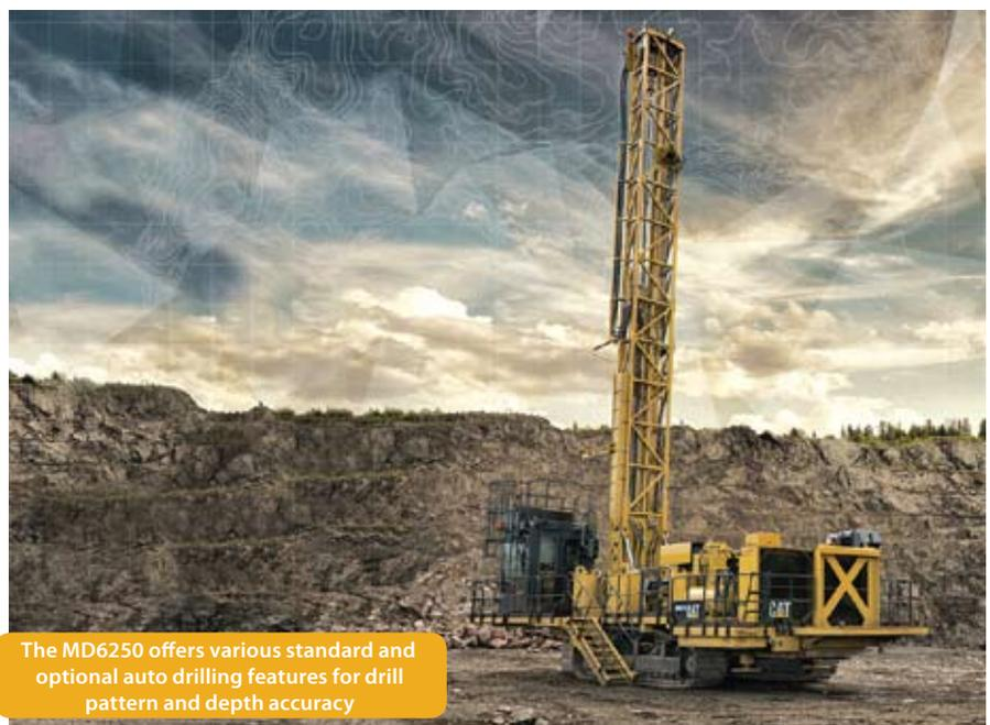
The MD6250 offers various standard and optional auto drilling features for drill pattern and depth accuracy
