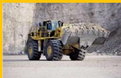
**"COMPARED WITH NON-ARM COMPONENTS, ARM-PROTECTED GET CAN LAST BETWEEN THREE AND FIVE TIMES LONGER IN HIGH-ABRASION/LOW-TO-MODERATE IMPACT CONDITIONS."**
