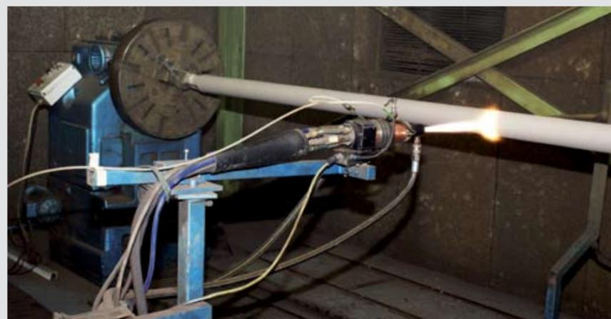
*During the final refurbishment phase, the HVOF process applies a coating to a hydraulic rod section in place of chroming within six to eight hours.*
